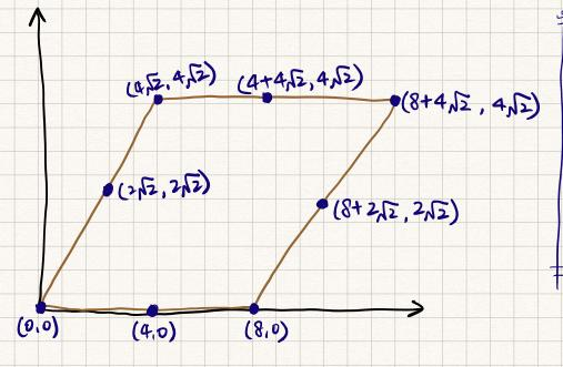
Even this one only has 4 vertices, try to find 4 more points to make it 8 nodes so that it can be used in the equations derived before
