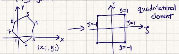
This mapping is done to easily integrate the strain energy and the work of the loads. J
